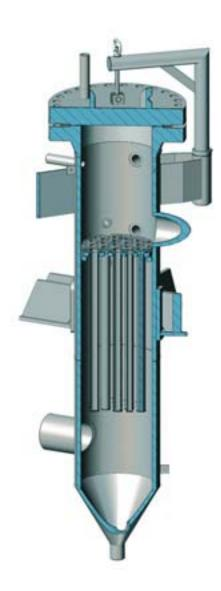
**Filtration:** The heat transfer oil to be filtered passes through the inlet nozzle of the filter casing and flows through the cylindrical filter elements from the exterior to the interior. The contaminants deposit themselves at the exterior surface of the filter elements and form a layer. The consequently cleansed filtrate flows out of the filter outlet as filtrate.
