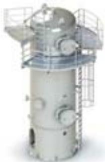
**Filtration:** The medium to be filtered flows through the interior filter layer from the top to the bottom, so that micro-particles are retained. The filter media consists of a filling with various layers of different material, e.g. filter sand and anthracite. This enables a superfine filtration of down to 1 µm. In order to optimize the separation process, a flocculent is frequently added to the filtrate.
