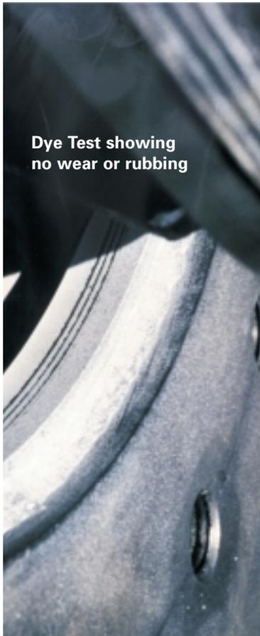
Dye Test showing no wear or rubbing
